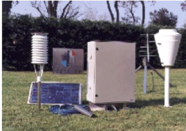
*The Hydrometeorological Data Collecting Platforms MED-HYCOS (DCP)*
